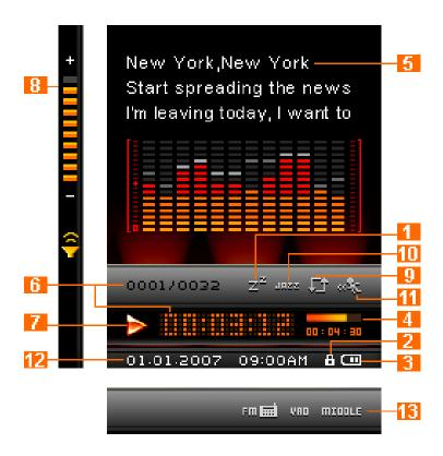
Figure 1. Color LCD Display
